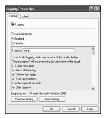
Figure 6-9 Configuring the installer logging options
