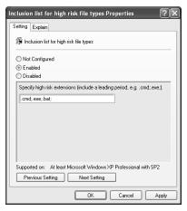
Figure 6-2 Overriding the default list with the file type inclusion list
