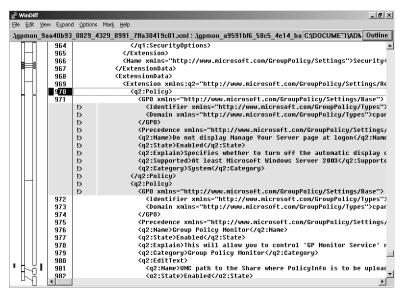
Figure 16-11 Displaying differences in RSoP reports through WinDiff
