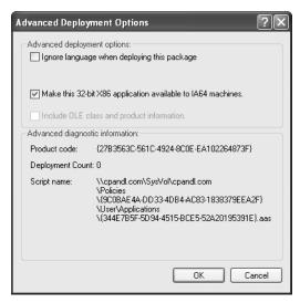
Figure 9-6 Configuring advanced software deployment options
