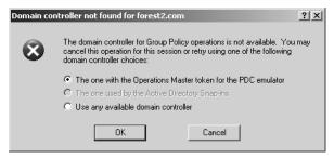
Figure 17-1 Error message indicating that the PDC Emulator is not available
