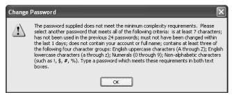
**Figure 5-9** Error message that occurs when a user types a password that does not meet the password policy requirements
