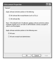
Figure 9-14 Working with enforcement options in Software Restriction Policy
