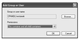
**Figure 2-15** Granting the permission to this container only or to the container and its child containers
